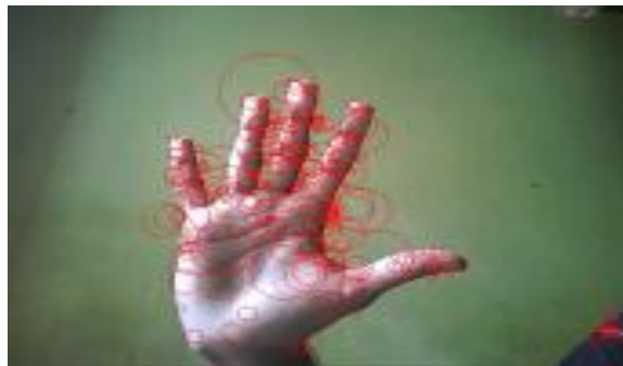
Figure 3: Shows interest points extracted from an image using SURF.
